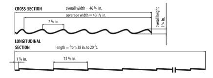
Fire Resistance: UL 790/ASTM E 108 Class A Fire Rating Impact Resistance: UL2218 Grade 4 Steel: ASTM A 792 Coil Coating: ASTM A 755 Florida Product Approval: FL41502
